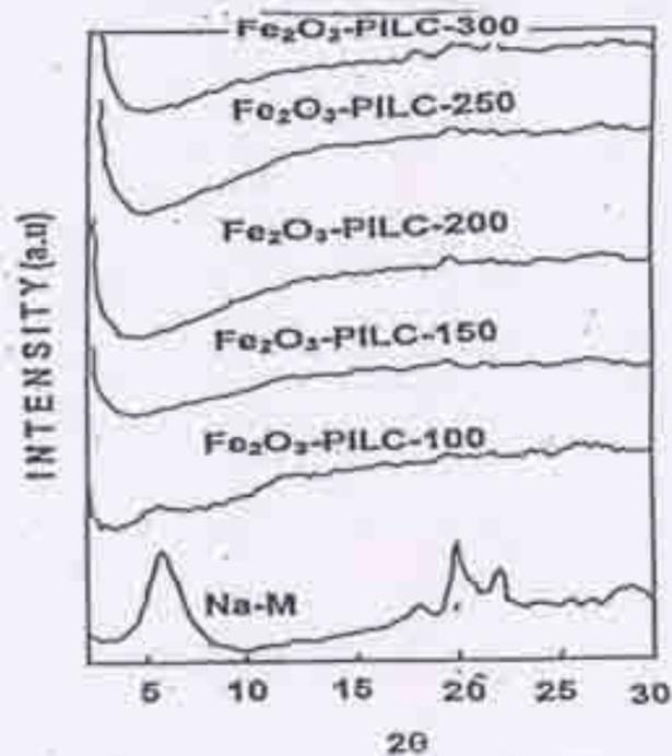
Fig.3. Xrd patterns of na-montmorillonite (hydrated), Fe<sub>2</sub>O<sub>3</sub>-pillared montmorillonite
