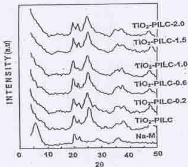
**Fig.2.** Xrd patterns of Na-montmorillonite (hydrated),  $\text{TiO}_2$ -pillared montmorillonite and  $\text{TiO}_2$ -pillared acid activated montmorillonite
