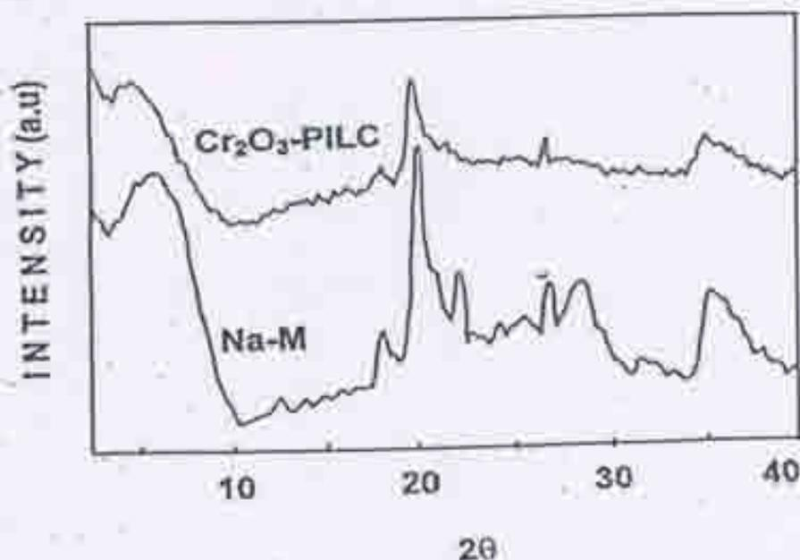
**Fig.4.** Xrd patterns of Na-montmorillonite (hydrated),  $\text{Cr}_2\text{O}_3$ -pillared montmorillonite
