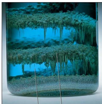
Blue color due to \text{Cu}^{2+} ions formed in redox reaction
