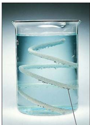
Copper wire in dilute \text{AgNO}_3 solution; after several hours
